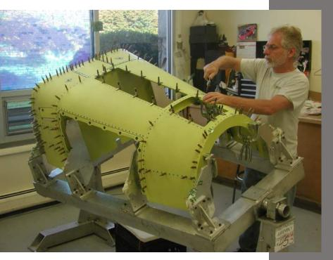
Fluid Mechanisms has a team of experienced assemblers skilled in installation of precision bearings, aerospace fasteners and metal bonding and sealing.
